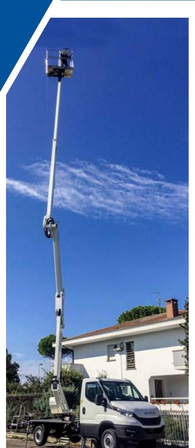
The GSR double articulated platform B200PX allows to reach a maximum horizontal outreach of 9 metres. This machine maintains the stabilization "in shape", with the result of being particularly compact.
