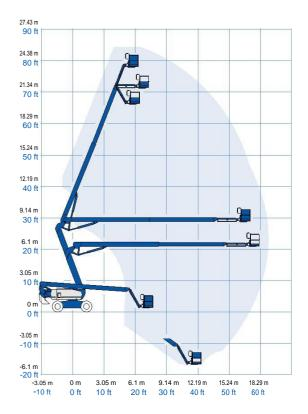
\* The metric equivalent of working height adds 2 m to platform height. U.S. adds 6 ft to platform height. \*\* In lift mode (platform raised), the machine is designed to operate on
