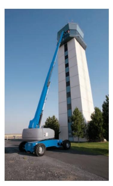
The horizontal outreach of the Genie® Super Boom™ line is among the industry's best at 75 to 80 ft (22.86 to 24.38 m), depending on the model.
