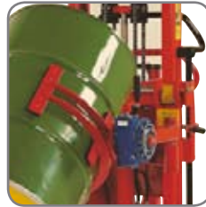
Quick shift makes it easy to replace the drum turner by other optional extras or forks.
