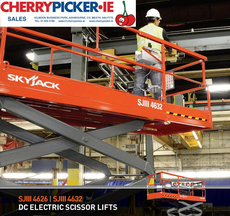
Skyjack's DC Electric Scissor Lifts offer high capacity and large platform areas, making them suitable for any on-slab application. Featuring variable speed rear wheel hydraulic drive, Skyjack 4626 and 4632 scissor models offer working heights up to 11.75 m and 25% gradeability.
